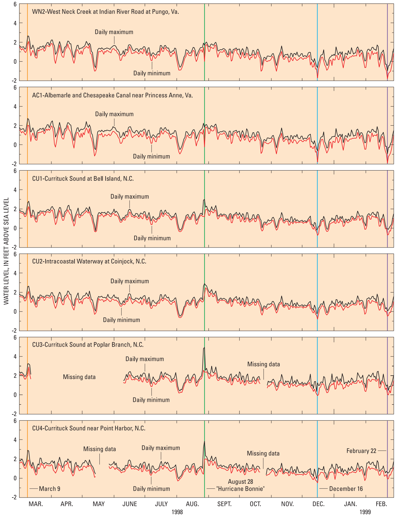
Figure 2. Daily maximum and minimum water levels at the Currituck Sound and tributary study sites from March 1, 1998, to February 28, 1999.
